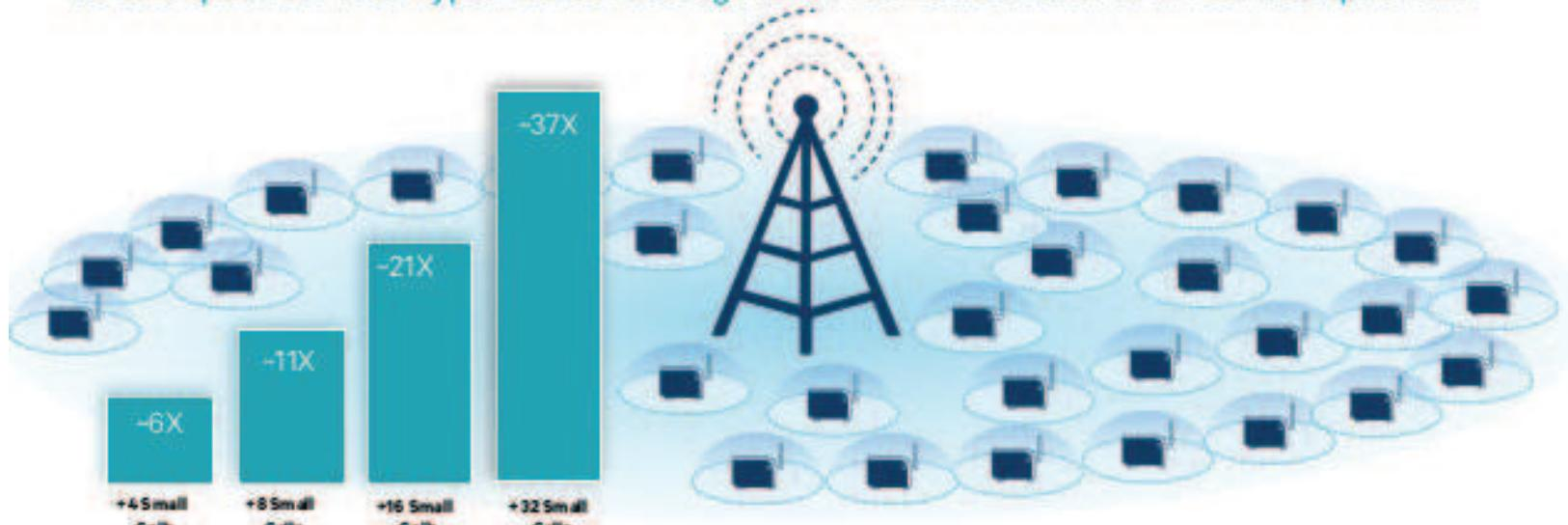
Assumptions: LTE Advanced with 256QAM enabled. Pico-type of small cell. 100MHz uplink/100MHz downlink scenario. 20dBs FDD uninterfered distribution scenario. Gain is median throughput improvement, thus baseline with macro only in 10MHz legal Get part of gains. Addition of 10MHz spectrum. Users uniformly distributed—a hotspot scenario could provide higher gains. Micro and outdoor small cells sharing spectrum (Co-channel).
