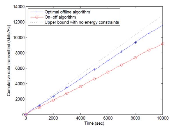
Improvement of optimal algorithm over an *on-off transmitter* in a simulation with truncated Gaussian arrivals.
