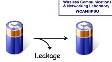
Optimal Policy: When total energy in an epoch is low, deplete energy earlier to reduce leakage.
